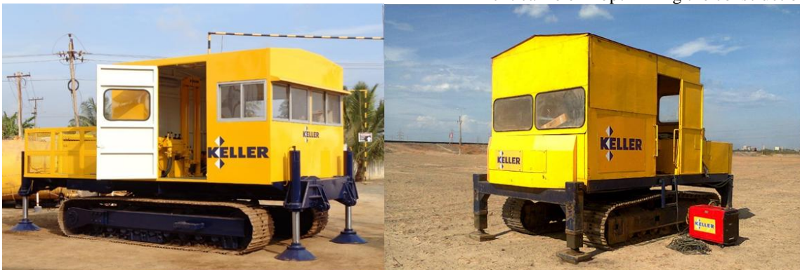
Figure 5: Electric Cone Penetration Testing Equipment
